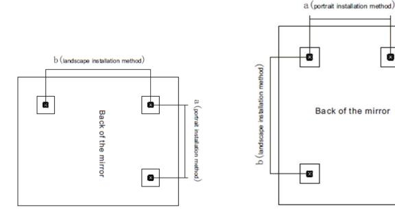
Mark this dimension on the wall, ensuring the holes are level, using a spirit level.
